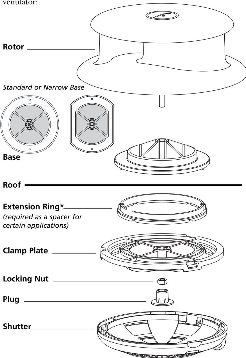
\*The extension ring is not usually required but can be used as a spacer between the clamp plate and the roof in situations where obstructions would prevent the clamp plate and shutter from fitting flush with the roof.
